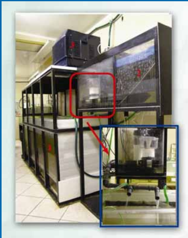
Recirculation water system (Moscow): 1 – Holding tank; 2 – Biofilter; 3 – Chiller.
